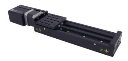
Zaber's X-LSQ-E Series products are computer controlled, motorized linear stages with a variety of lead screw pitches and travels. The built-in motor encoder allows closed-loop operation and slip/stall recovery features. They are stand-alone units requiring only a 48 V power supply, included with the kit version.
